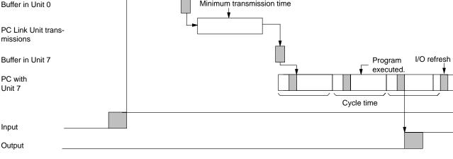
The equation for minimum I/O response time is thus as follows: Response time = Input ON delay + Cycle time of PC of Unit 0 + Minimum transmission time + (Cycle time of PC of Unit 7 x 2) + Output ON delay Inserting the following values into this equation produces a minimum I/O response time of 149.3 ms.
